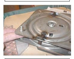
Next, insert the four shorter bolts up through the slotted holes of the base side of the swivel.
