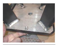
Align the base with the four bolts. If your base has an extended footrest, make certain that the extended portion faces the front of the chair. Using two 7/16" wrenches, tighten these four bolts and nuts securely.
