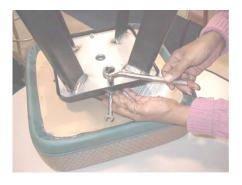
Place chair on bench, up side down. Using two 7/16" wrenches, remove the four bolts holding the base to the swivel. Remove the base and set aside, right side up, away from the work area.
