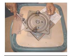
With one hand, rotate the swivel until the bolts which attach it to the seat are visible. With the other hand, using a 7/16" wrench, remove these four bolts. Remove old swivel mechanism.
