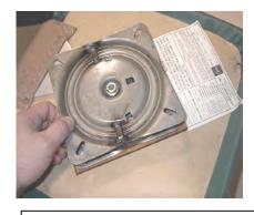
Position new swivel mechanism over threaded inserts on seat bottom, making sure that the side stamped "front" on the swivel faces one of the front corners of the chair seat.
