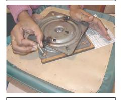
Insert the four longer bolts through the mounting holes in the swivel and into threaded inserts in the seat bottom. Note that the rear bolt also passes through the back plate. Tighten all four bolts securely.
